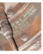
Before restoration, the data plate of the Sh.IIIa was covered with a fine layer of rust (left). **Refurbishing the** engine's crankcase (below) was a demanding task. "It was a long day at work," remembers Genchi. "I was very tired."
