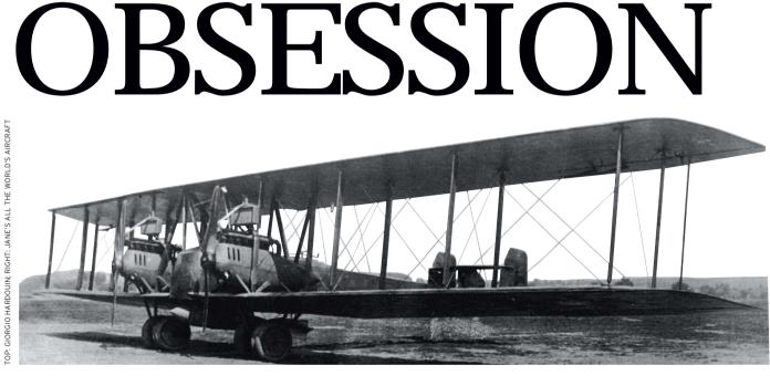
**Opposite:** Giuseppe Genchi, who found a trove of engine parts at the University of Palermo, spent countless hours restoring an 11-cylinder rotary engine from World War I. The Friedrichshafen G.V bomber prototype (below) was powered by two Mercedes D.IV engines. Genchi restored a D.IV for the university
